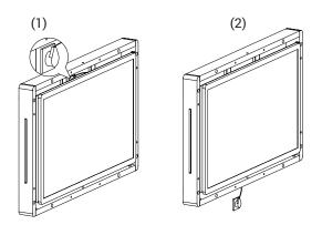
Two possible ways to mount the product to the wall. (1) Power socket within frame. (2) Power socket outside frame.
